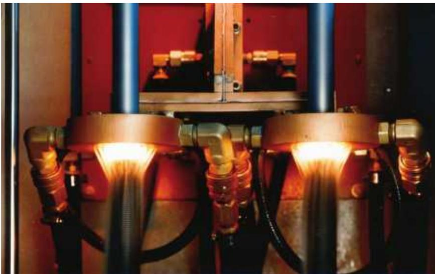
Fig. 1. Dual shaft induction scanner
