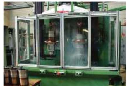
**Fig. 6. Unitized machine with two independently operated heat stations and high-speed, servo-driven scanning assemblies for induction hardening the ID of gray iron cylinder liners. Production rate is 50 liners/h with a 0.8 mm (0.03 in.) case having 47-49 HRC as-quenched hardness. Courtesy of Inductoheat Banyard Ltd., Dorset, UK.**
