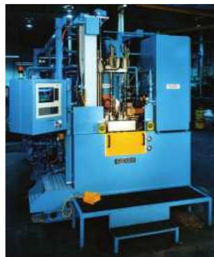
**Fig. 4. Compact system for hardening cast iron camshafts. Courtesy of Inductoheat Inc.**
