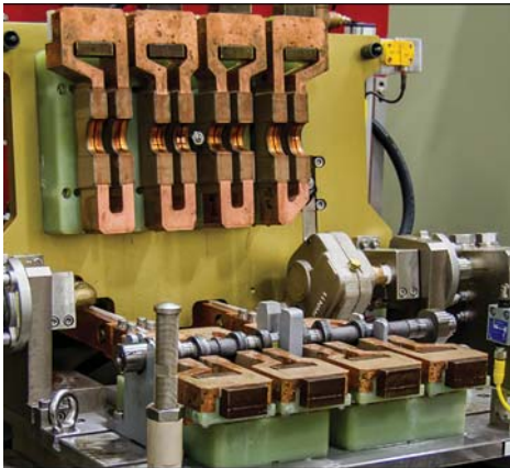
Fig. 3. CamPro™ machine utilizes patented non-rotational hardening technology (SHarP-C™ technology)
