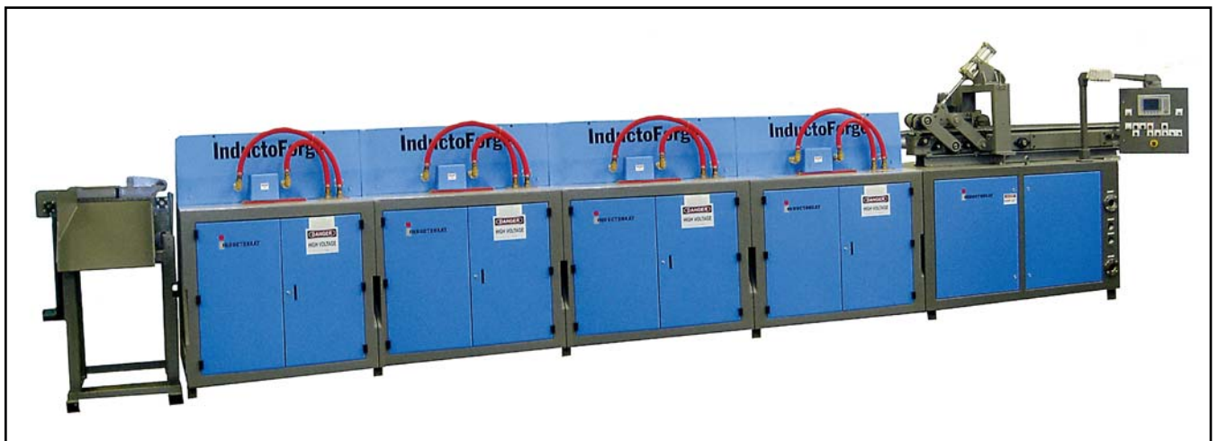
FIGURE 5: InductoForge modular induction bar and billet heating system
