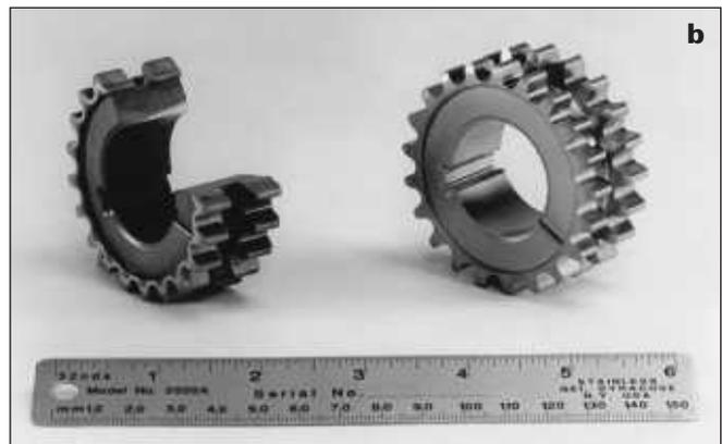
*Fig.16. A unitised induction system (a), capable of providing both CSFC and PSFC gear hardening, is used to harden the double sprocket shown in (b).*
