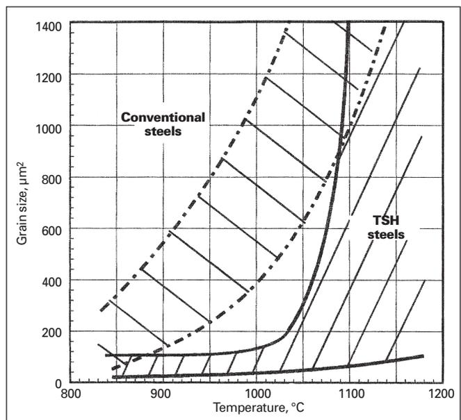
Fig.22. Grain growth for TSH steels versus that of conventional grades<sup>20</sup>.
