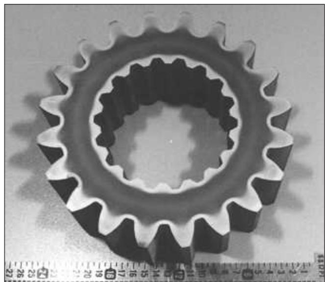
Fig.23. Induction heat-treated gear made from TSH steel.
