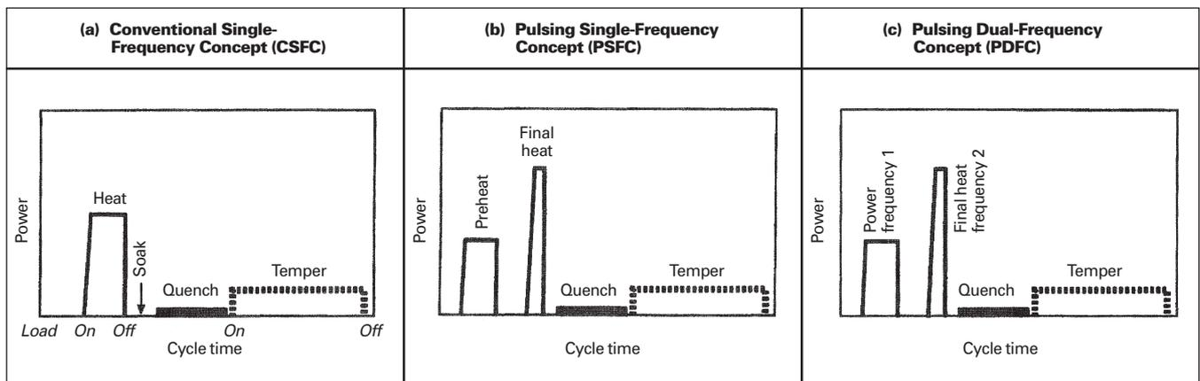
Fig. 13. Concepts of gear hardening by induction.
