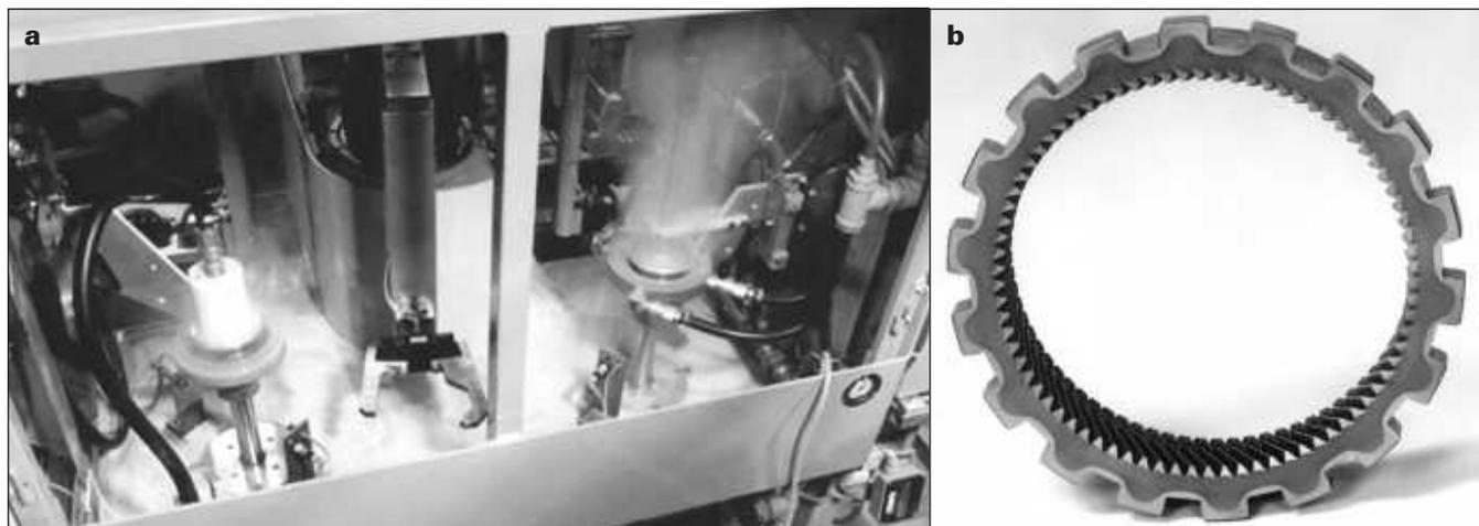
Fig. 14. (a) Equipment used to harden OD and ID of gears such as that in (b). (Courtesy of Inductoheat Inc.).
