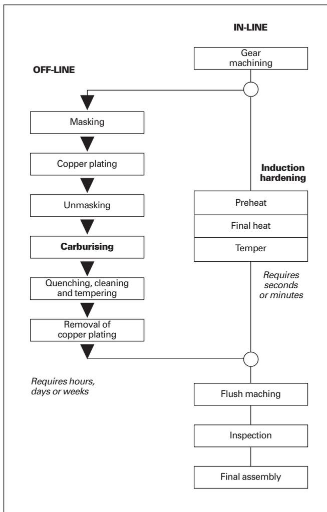
Fig.20. Steps required for carburising compared with those for induction hardening<sup>18</sup>.
