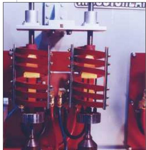
Fig. 1 — Induction machine for brazing tips to tool bits for use in the mining industry. With multiturn coils such as these, the electromagnetic field distribution can be tailored by varying the coupling gap and/or the distance between coil turns. Photo courtesy Inductoheat Inc.
