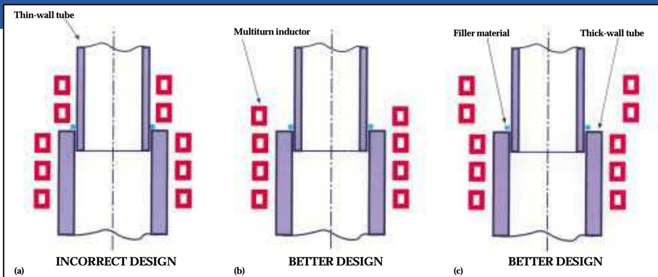
Fig. 3 — This example involves joining similar materials having different cross sections. (a) A uniform coupling gap results in overheating of the thin-wall tube. (b and c) Better designs concentrate heat into the more massive thick-wall tube, producing reasonably uniform heating.
