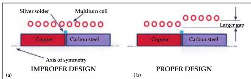
Fig. 2 — Brazing dissimilar materials requires a nonstandard coil configuration. (a) A uniform coupling gap overheats the carbon steel and underheats the copper in this example. (b) A larger coupling gap on the steel portion of the joint provides a more uniform heating pattern for both materials. (Ref. 1)
