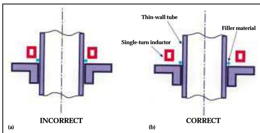
Fig. 4 — Coupling gaps also can be changed to accommodate differences in component shape and mass, as well as thickness. (a) Overheating of a thin-wall area, due to a relatively small mass and incorrect placement of the inductor. (b) Repositioning the induction coil ensures uniform heating of the entire joint area.
