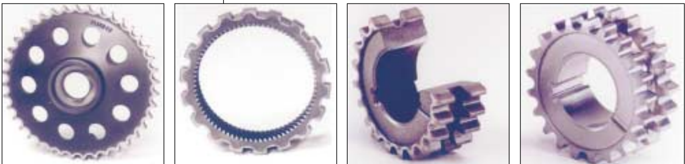
Fig. 1 — External spur and helical gears, worm gears, and internal gears, racks, and sprockets are among those that typically are induction hardened (examples shown here). Bevel, hypoid, and noncircular gears are rarely heat treated by induction. (Courtesy Inductoheat Inc.)
