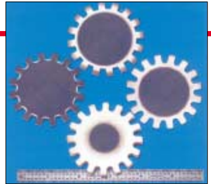
Fig. 2 — A variety of hardened patterns can be obtained by varying induction heating time, frequency, and power. (Courtesy J. LaMonte, Inductoheat Inc.)
