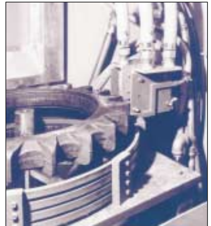
Fig. 4 — Induction spin hardening of a large gear. The heated gear will be quenched by immersion. (Courtesy Inductoheat Inc.)
