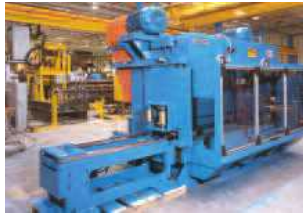
Alpha 20 cm shear for cutting tube for hydroform applications at 100 M/min
