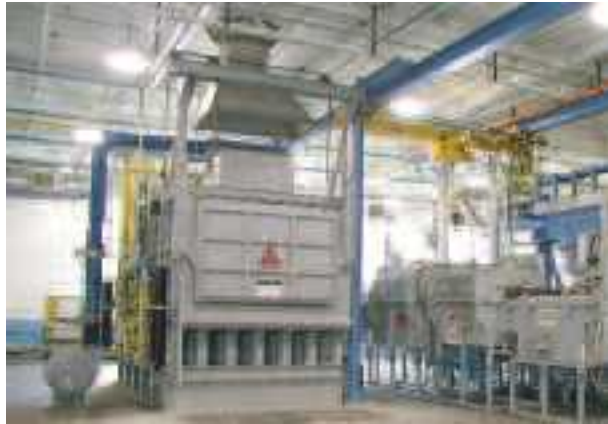
1,800 kg/hr integrated aluminum treatment & casting line
