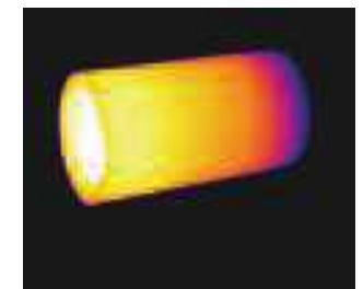
Stress relieving before threading of premium casing and tubing
