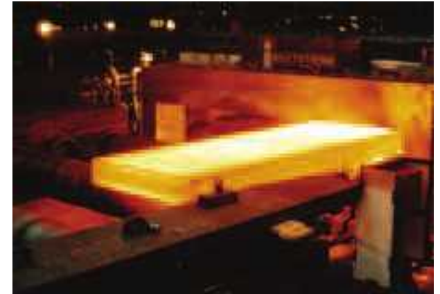
Induction reheating of slab prior to rolling
