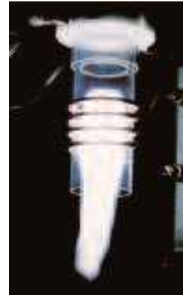
Thermatool HF Plasma Generator
