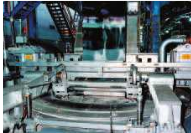
Coreless coating pot for a continuous strip line
