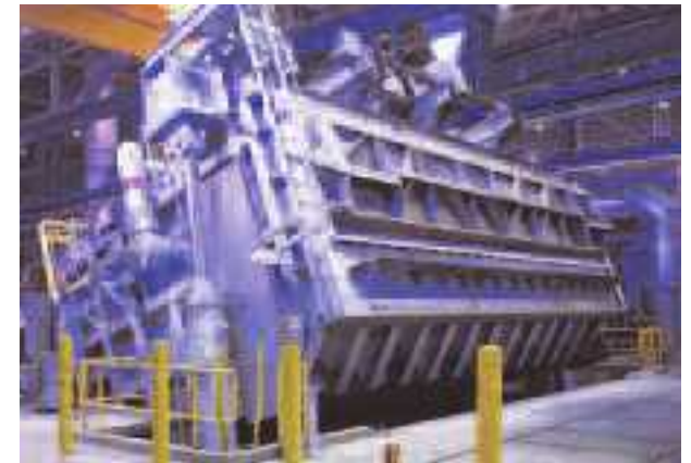
110,000 kg capacity aluminum tilting holding furnace
