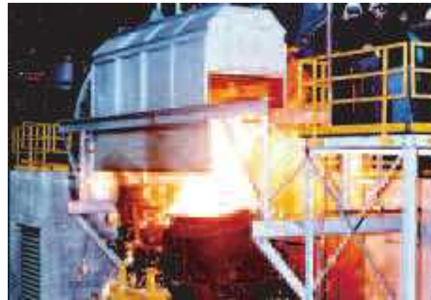
Three 16,500 kW 20T furnaces pouring 80T iron/hr
