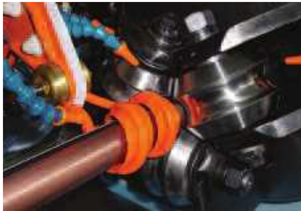
High-speed induction tube welding
